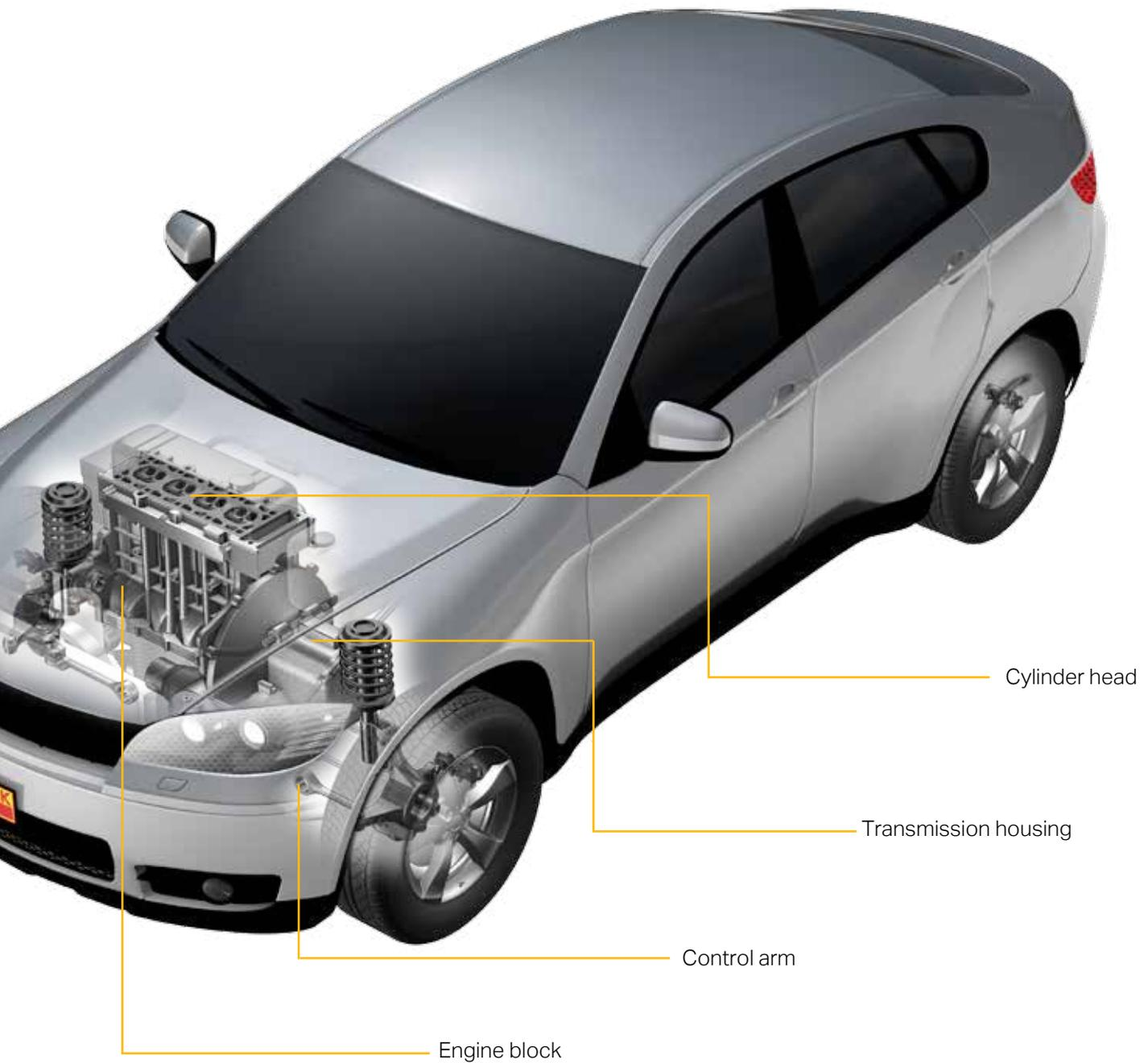
Exchanging traditional steel components with aluminum components provides up to 50% weight reduction
